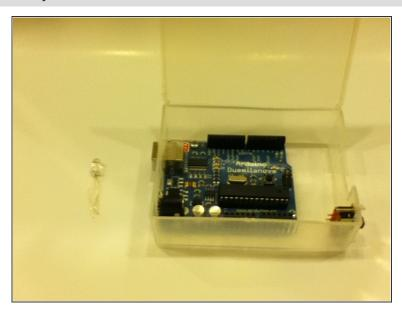
Now for the physical parts. As you can see to the left, all you need for this first project are an LED and an Arduino. The box and switch are part of my Arduino housing and aren't required.
